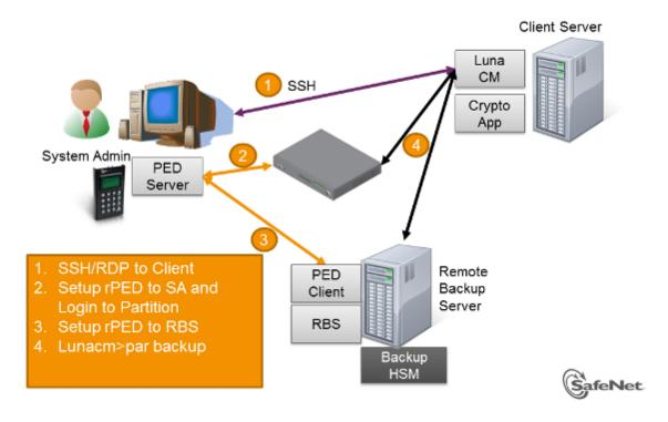
Backup is controlled via the lunacm:> command line. As a system or security administrator, you choose which computer is to run lunacm:> to accomplish the backup/restore operation.
