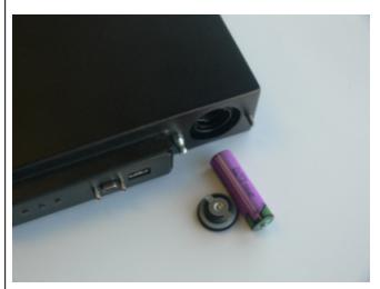
Remove the battery from its packaging and align it at the opening of the Luna G5 battery compartment. The battery has a "+" sign near the end with the raised nub/bump. The flat end of the battery is the negative pole (-).
