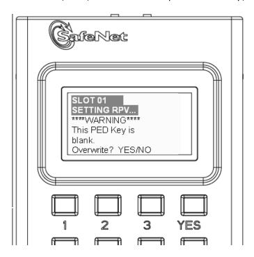
Answer [YES] so that the HSM can create an RPV and transfer it to the PED, where it is imprinted onto the blank PED Key that you have inserted. If you invoked M of N, then the PED will prompt you to continue inserting orange PED Keys for imprinting with portions of the secret until you have imprinted quantity N of them.
