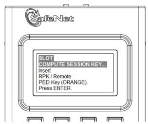
2. Insert the orange PED Key that you brought from the HSM to the remote PED, and press [Enter] on the PED keypad.
