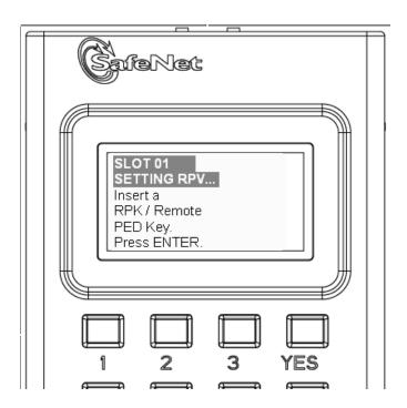
Do as prompted, inserting an unused PED Key into the PED's key slot (top-right of the PED), and press [ENTER].
