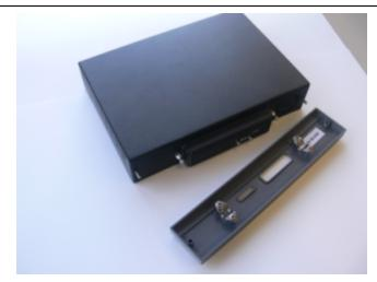
Begin by removing the front face-plate. It is held in place by two spring clips. Grasp the face-plate firmly and pull to disengage the clips. Set the face-plate aside.
