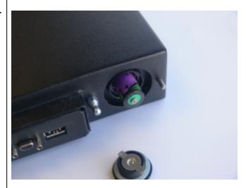
Insert the battery, negative end first. The positive end (+) should protrude. The compartment is spring-loaded.
