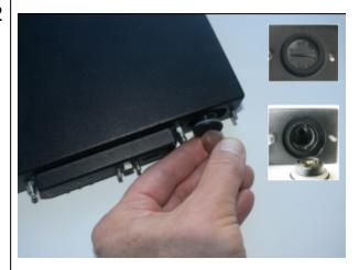
The battery compartment is to the right as you face the unit. The compartment cover is circular and has both raised dots and a recessed slot. Use finger-pressure against the dots, or the edge of a coin in the slot, to twist the battery compartment cover ¼ turn in a counter-clockwise direction. The cover should fall out easily.
